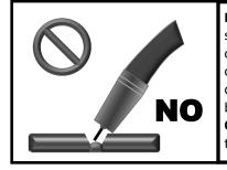
**Problem:** Gun is not being held vertical from side to side. Wire is not being directed to the center of the puddle. This concentrates heat on one side of the joint and results in poor fusion on the neglected side. It also can create more buildup on one side of the joint than the other. **Correction:** Hold the gun so that the angle of the neck stands perpendicular from side to side.
