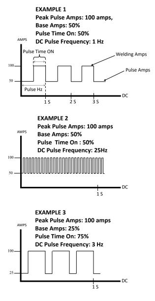
the standard unit "Hertz." Simply, it is the number of pulses per second that occur. Pulse frequency controls the arc constriction and also helps with heat management.
