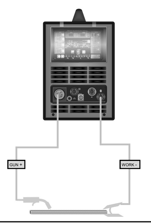
\*The feeder connection located under the spool cover must be located on the positive terminal. MIG requires that the gun be used with a positive polarity.
