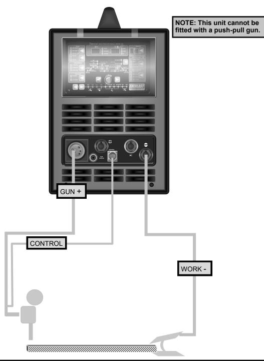
\*The feeder connection located under the spool cover must be located on the positive terminal. MIG requires that the gun be used with a positive polarity. Keep in mind that if the gun is used with steel flux-core wire the work connection must be positive and the gun connection must re-connected negative under the spool cover.
