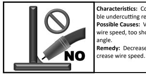
Characteristics: Concave weld, poor filling, possible undercutting resulting in weak weld. Possible Causes: Voltage too high, not enough wire speed, too short of wire stick out, wrong gun angle. Remedy: Decrease voltage, use push motion, in-
