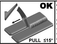
**Correct Technique:** The gun is angled toward the back of the weld when traveling forward. This angle should not exceed 15 degrees. This provides a narrower but more deeply penetrating weld. Use this method when Flux Core wire is being used. Use this method where the unit may be reaching its maximum welding capacity. Not for use with Aluminum wire.
