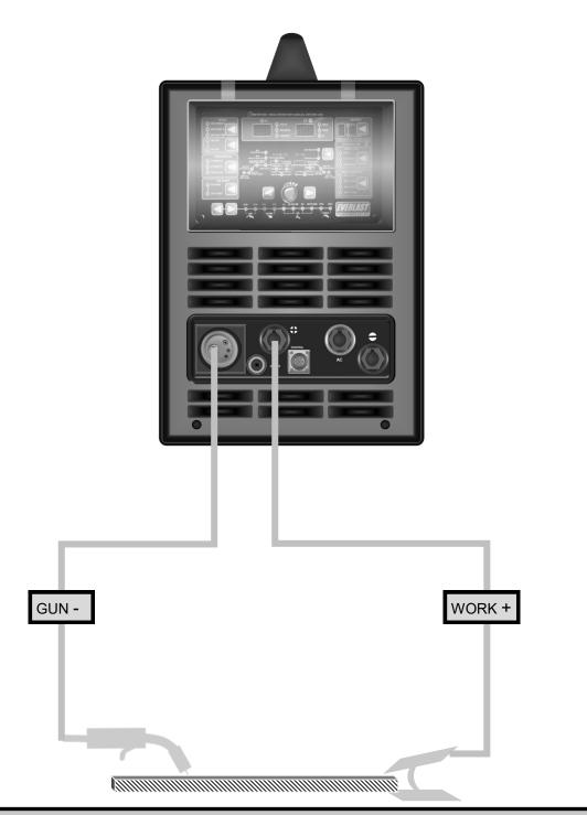
\*The feeder connection located under the spool cover must be located on the negative terminal. Flux-Core wire requires that the gun be used electrode negative (EN) in most cases. Consult the wire manufacturer recommendations as the final authority . Dual shield wire is run
