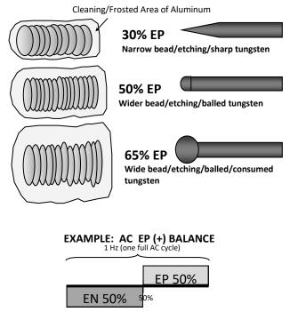
Standard transformer welder balance: 50% EN/EP Balling tungsten, light penetration, wide cleaning area.
